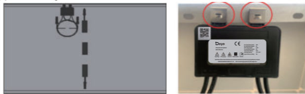
b. Diagram of the location of the optimizer component c. Optimizer fixed diagram
