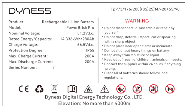
Figure 1-1 Battery Module Label
